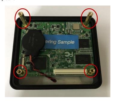
3. Fasten the spacer on the motherboard by the two remaining 9mm hex standoffs.
