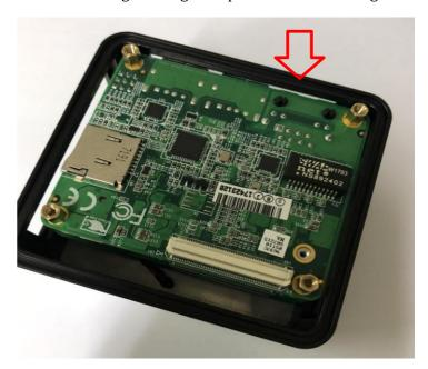
7. Place the bottom base on top of the stacking housing and tighten this with the M2.5\*6 screws that are packaged with the main housing.
