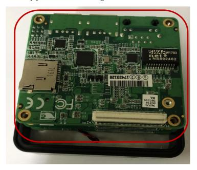
5. Use the four hex standoffs (5.5mm, silver) that are packaged together with main housing accessory package to fasten the stacking board.
