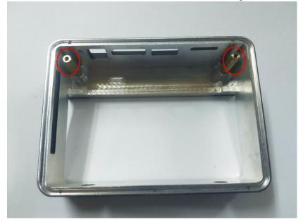
3. Assemble the heatsink top into the middle base.
