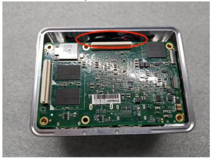
7. Fasten UP core Board to the top cover with the M2.5\*5 hex standoffs (thread nuts)
