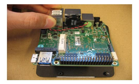
6. Fasten the PCB with the top cover by the hex standoffs through the threads nut on the top cover.
