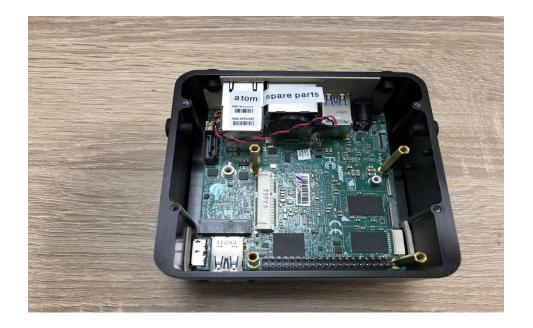
8. Fasten the bottom plate with PCB by screws x 4pcs Fasten the bottom plate with top cover by screws x 4pcs.
