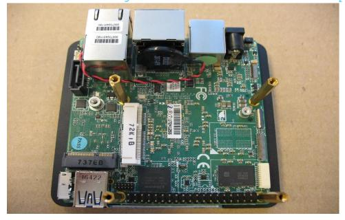
7. Place the board and Top heatsink into the middle case, check well with the 4 sides that they exactly match the IO sides.
