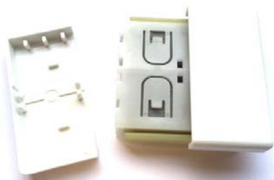
Clip both rockers onto the PTM module
