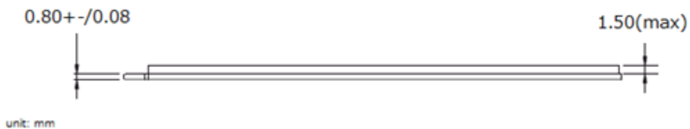
Figure 3-1: Side View of SSD
