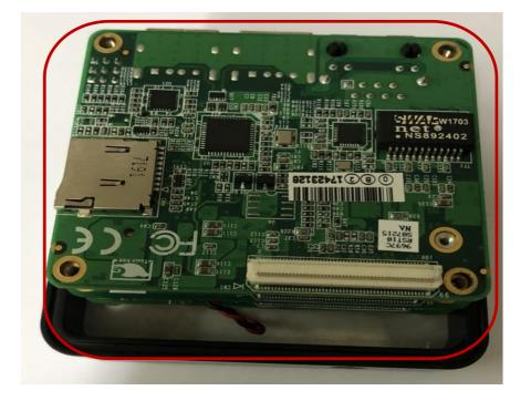
4. Carefully place the UP stacking board on the four hex standoffs.
