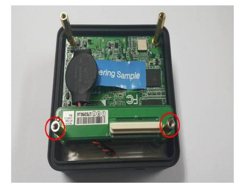
3. Fasten the spacer on the motherboard by the two remaining 9mm hex standoffs.
