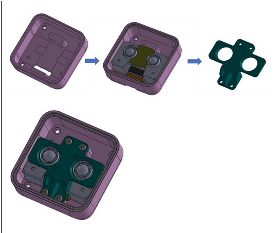
Figure 7-15. Stereo Depth Module Mid-Mounting – D401
