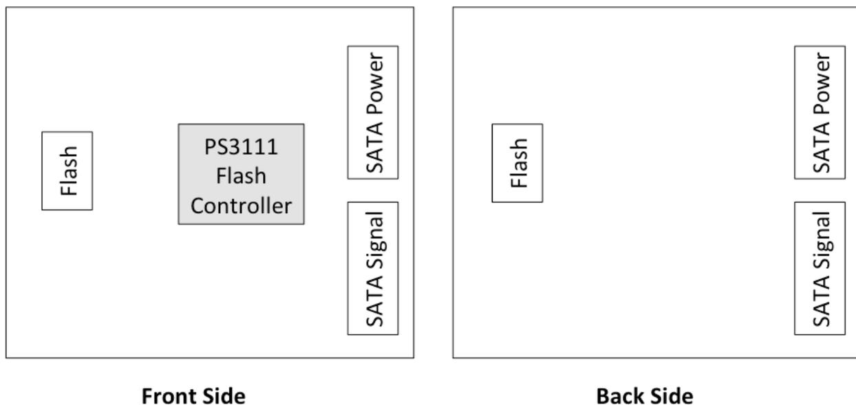
Figure 1-2 PS3111 M.2 2242 Product Block Diagram
