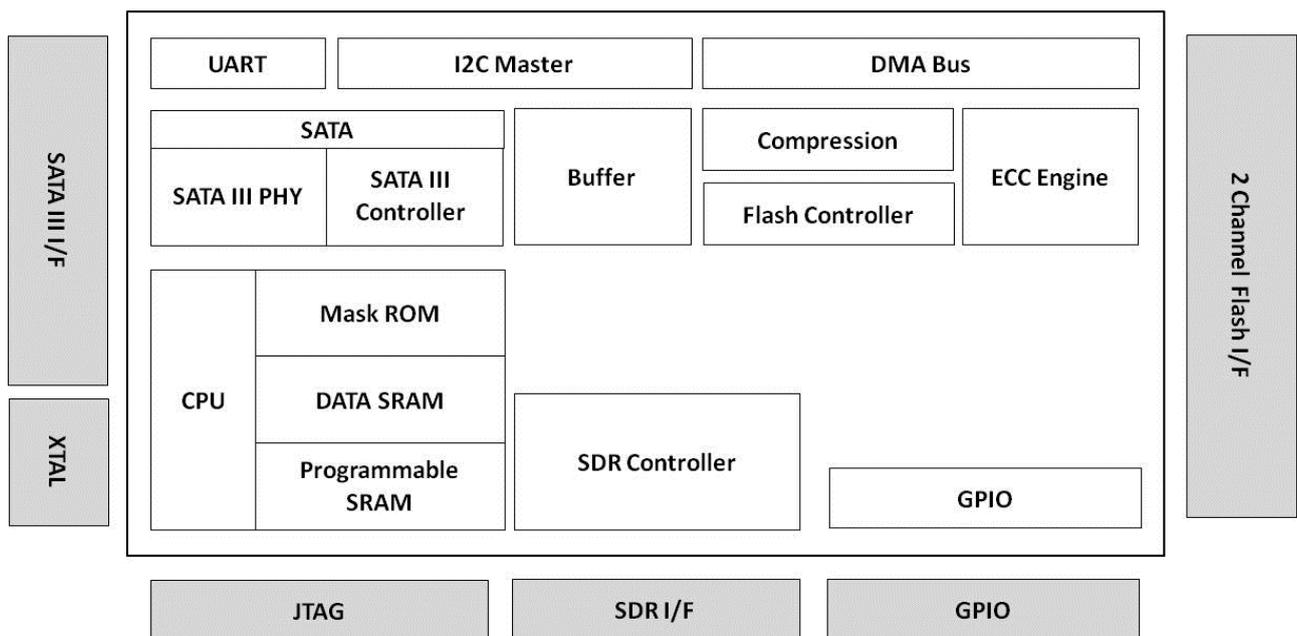
Figure 1-1 PS3111 M.2 2242 Controller Block Diagram
