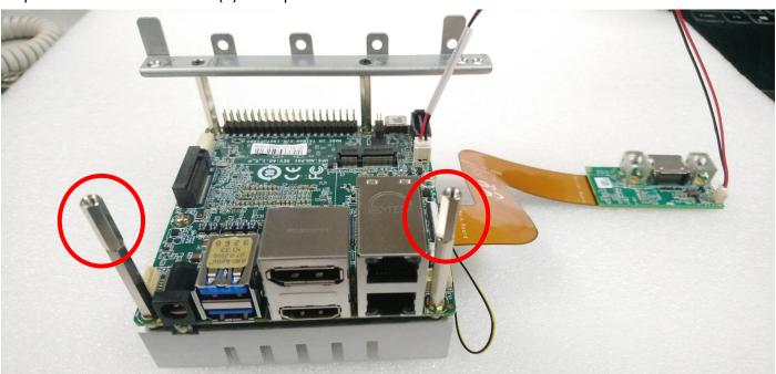
Step 7: Affix and lock the Two (2) sliver screws to the HDMI IN carrier board.
