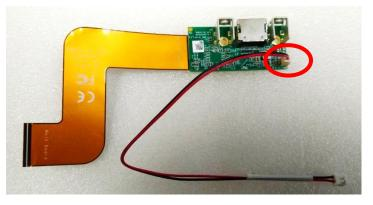
Step 4: Unlock the main board FPC connector, the plug the FPC cable and power cable into it.
