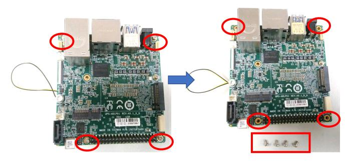
Step 2: Affix and lock the four (4) pillars to the board in the following sequence.
